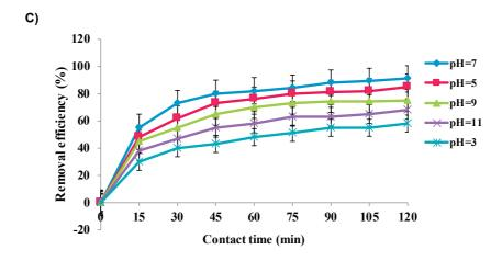
Figure 4. Impact of parameters on adsorption of diazinon onto PLA/Fe<sub>3</sub>O<sub>4</sub>@ $\beta$ -CD nanofi brous nanocomposite . A) Effect of adsorbent dosage and B) Effect of initial concentration of diazinon. C) Effect of initial pH on the adsorption of diazinon onto PLA/Fe<sub>3</sub>O<sub>4</sub>@ $\beta$ -CD nanofibrous nanocomposite .xlsx
