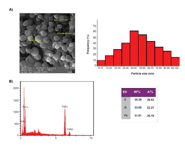
Figure 1. Characterization of Fe<sub>3</sub>O<sub>4</sub>@β-CD nanoparticles. A) The SEM image and the size distribution histogram B) EDS analysis.
