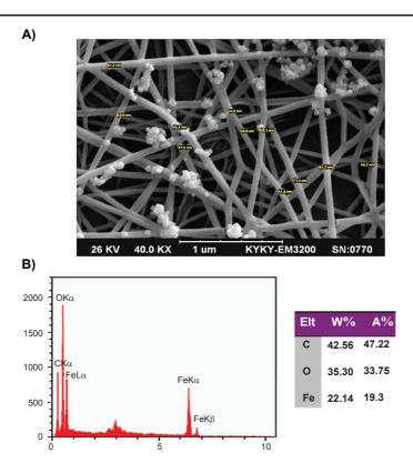
Figure 2. Characterization of PLA/ Fe<sub>3</sub>O<sub>4</sub>@β-CD/ F. angulate.extract nanofibrous nanocomposite. A) SEM images, B) EDS analysis.
