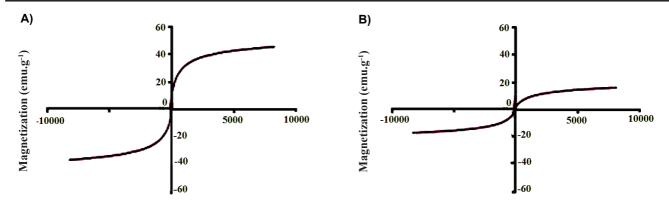
**Figure 3.** The magnetic hysteresis loop curves .**A**) Fe<sub>3</sub>O<sub>4</sub>@β-CD nanoparticles and **B**) PLA/ Fe<sub>3</sub>O<sub>4</sub>@β-CD/ F. angulate extract nanofibrous nanocomposite.
