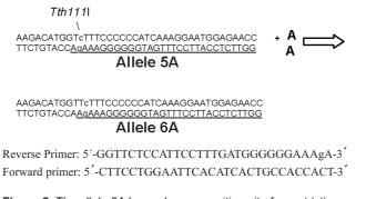
**Figure 2.** The allele 5A has only a recognition site for restriction endonuclease Tth1111 (3'-CAGN-5').
